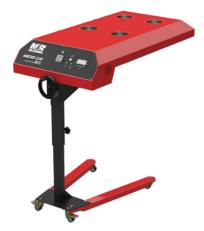
Ancho is M&R Global's versatile freestanding quartz flash cure system. It has a universal design that can fit most brands' presses. An adjustable sensor switch can be positioned on either side of the flash cure unit, activating the flash when the printing pallet approaches. It uses medium wave filament quartz lamps and flash cure duration can be controlled by an analog timer.
